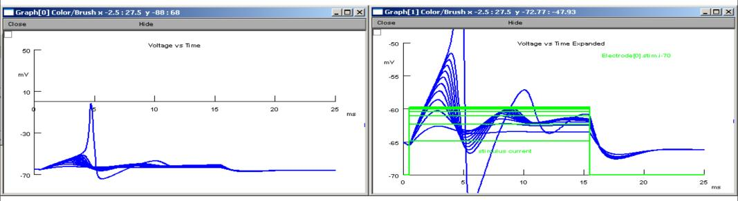
At 20 deg Celcius, the critical current threshold is at I = 10.242 nA. Much higher than the current required to generate an action potential at 2 deg Celcius.
