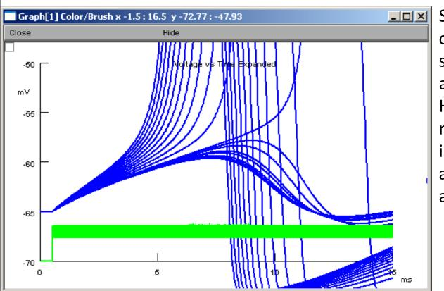
Side note: as the amplitude of the current increases, the action potential shifts to an earlier onset by a smaller amount of time. This occurs because HH model is a non-linear system. If the neuron only had leak channels, the shift in the onset time will change equally along all change in values of the current amplitude change.
